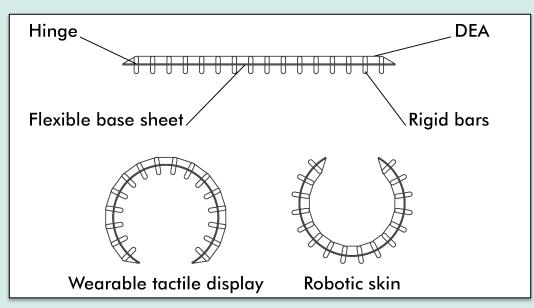
We are developing a new version of the display with a flexible base sheet, suitable for wearable devices. A further application of the device could be soft robotic skin, so that the robot would be able to feel if a person touched it, but the person would also get some tactile feedback from the robot e.g. about the state of the robot or the current danger level.
